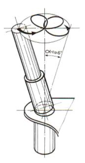
Because the improved, revolutionary technique with cycloidal movement of the peen replaces the current hammering, rolling and wobbing (orbital – spin) techniques or riveting and our radial riveting system produces a better rivet fusion
