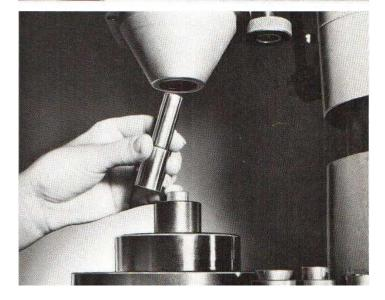
The riveting peen does not turn in rotation. It is held in place by a permanent magnet and can be slide in and out by hand.
